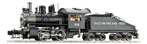
AML is proud to offer the famous B&O 0-4-0 of the Baltimore Waterfront. Four switchers were built in 1912 by Baldwin for the B&O. Initially constructed as saddle tank engines, some were given tenders in later years. The diminutive size and short wheelbase were required to handle the tight curves of these lines.
